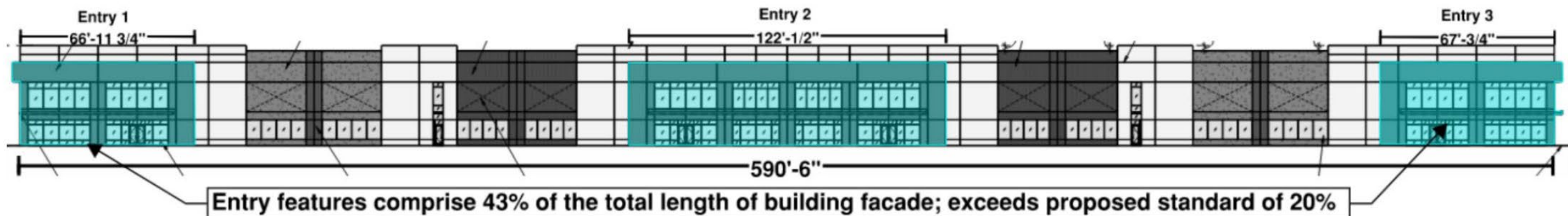
Figure 3: Entry feature length requirement
